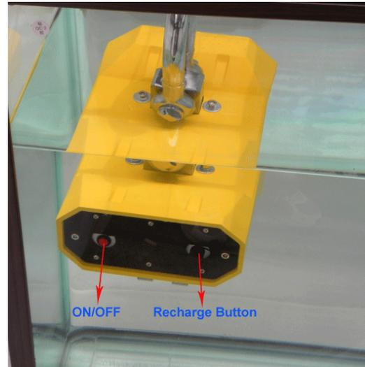
**Water proof crane scale OCS-SL is re-equip model based on ordinary crane scale OCS-SL. We take out the two keys (ON/OFF, TARE) of the front panel, and put the ON/OFF key on the back panel. On the back panel, the black button is used for recharging battery. The TARE function can be achieved through the TARE key on the remote control. All other function is just as same as ordinary model, please refer our user manual OCS-SL**
